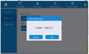
Fig. 5-6 Fault clearance
