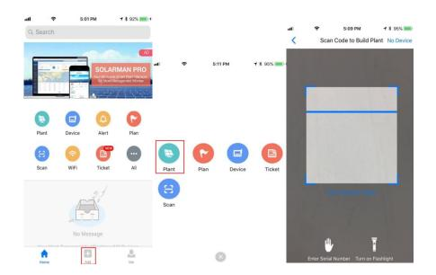
Method 2: click the [Plant] icon first to enter the plant list, then click [+] in the upper right corner to add the plant, then scan the serial number of the stick logger.
