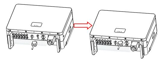
The RJ45 plug for electric meter communication and digital input is inserted into the COM2 connector, the RJ45 plug for DRM communication is inserted into the COM3 connector (only for Australian configuration).
