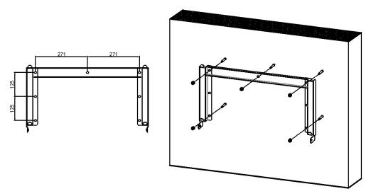
4. Attach the inverter to the wall mounting bracket. Screw the inverter to the wall mounting bracket on both sides using the M5 screws provided. Tighten the screws and make sure that they are securely in place.
