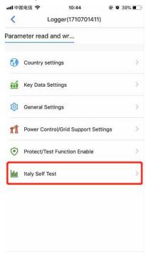
4. In the self-test page, select the 'Italy Self Test Setting' and enter the page of selecting the self-test item.
