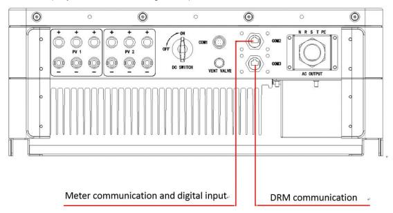
The enlarged image of the meter communication interface and DRM communication interface is as shown below:
