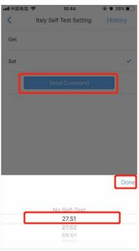
6. After successful sending, go back to Italy self test page and select the item of Italy self test.
