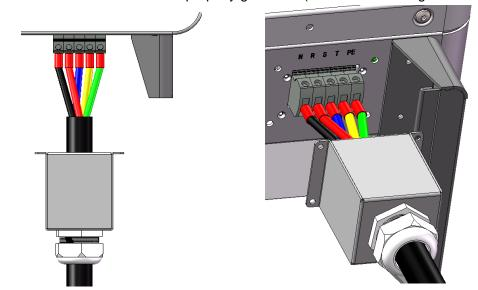
3. Combine the shell and the AC terminal of inverter with the combination screws M4  $\times$  10.
