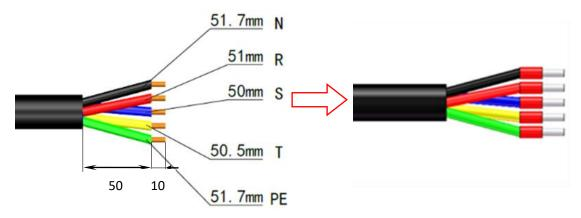
2. Fix L1,L2,L3,N and PE wires to the corresponding AC terminals with a screwdriver and ensure that the PE wire is properly grounded (As shown in the figure below).
