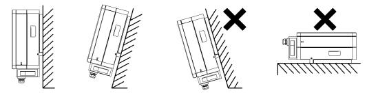
In order to maintain sufficient ventilation, when installing the inverter a minimum clearance of 30 cm at the sides and 50 cm at the top must be maintained. Operation and reading are made easier by installing the inverter with its display at eye level and by keeping a distance of 100 cm from the front. All cables are routed to the outside through the underside of the enclosure, therefore a minimum clearance of 50 cm must be observed here.
