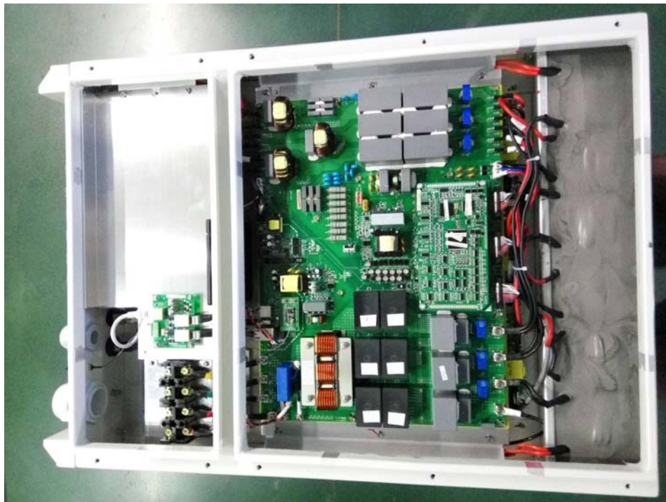
Photo 8 Inside structure view—AC connective terminal (alt.)
