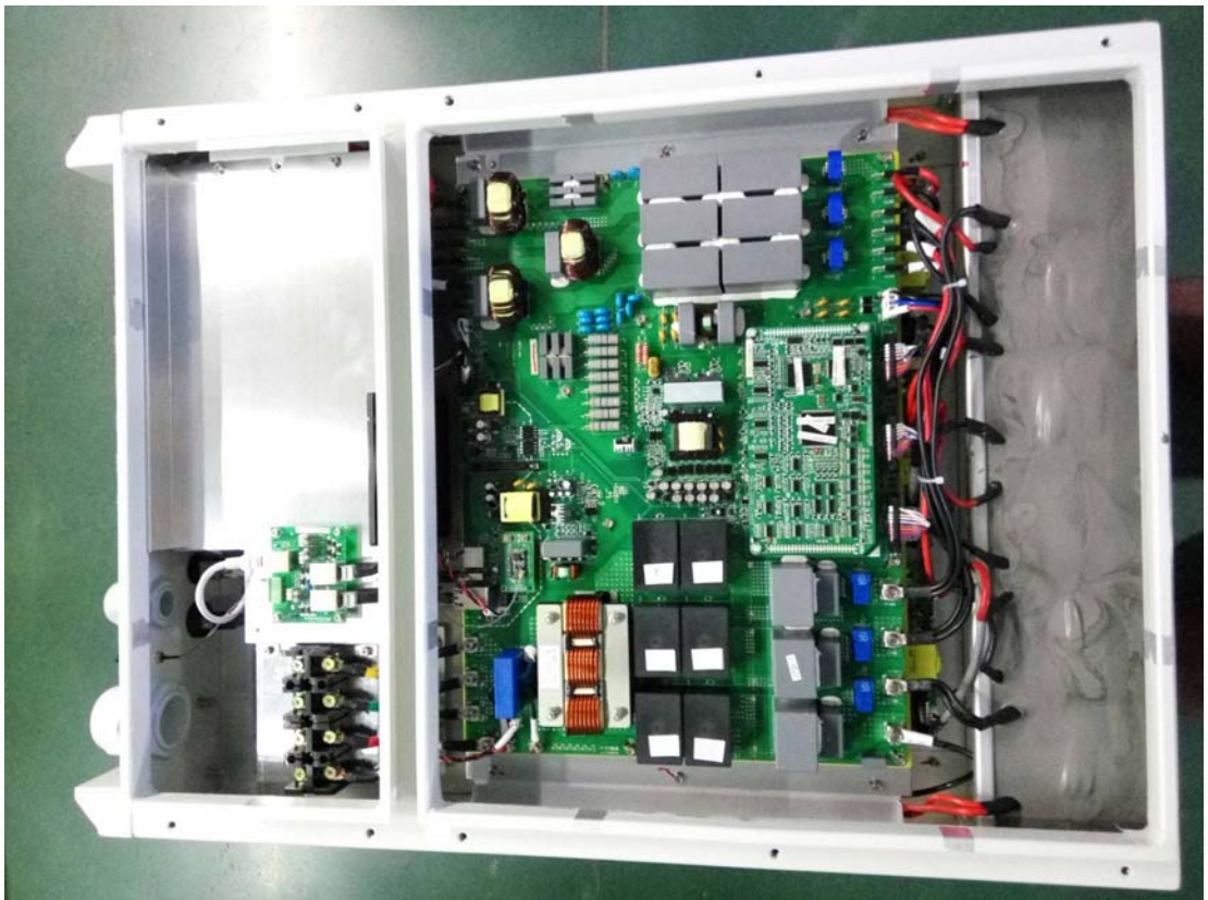
Photo 8 Inside structure view—AC connective terminal (alt.)
