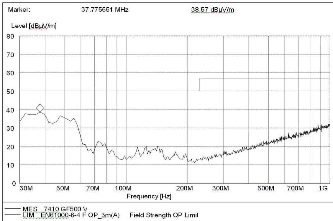
2. Electromagnetic radiation disturbances, max peak detector, antenna polarization: Horizontal
