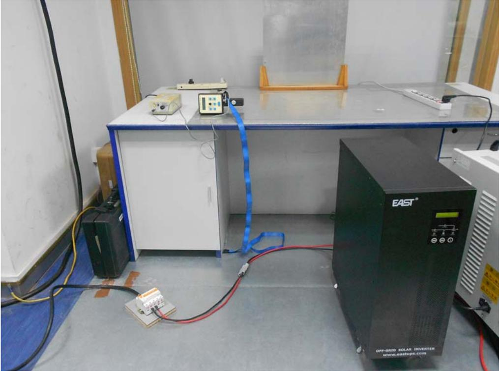
**5. Radiated, Radio Frequency Electromagnetic Field Immunity Test (below 1GHz)**
