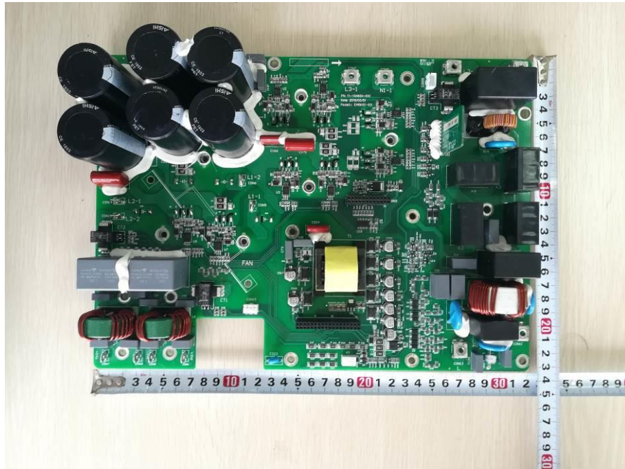
Figure 11. Component side view of Main board for model: EA3KSI-D, EA3.68KSI, EA4KSI, EA4.6KSI, EA5KSI, EA6KSI, EA7KSI
