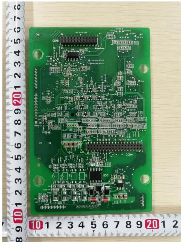
Figure 14. Solder side view of Control board
