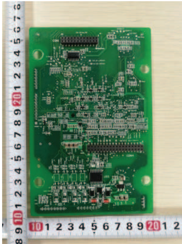
Figure 14. Solder side view of Control board
