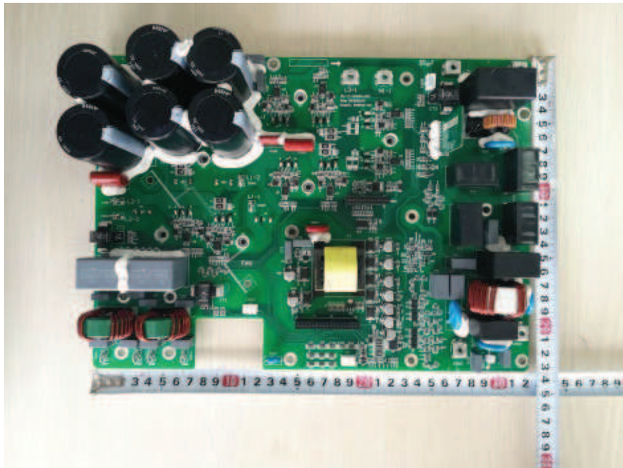
Figure 11. Component side view of Main board for model: EA3KSI-D, EA3.68KSI, EA4KSI, EA4.6KSI, EA5KSI, EA6KSI
