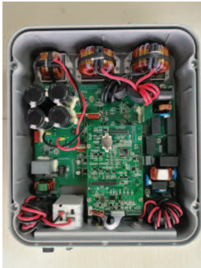
Figure 4. Internal view-1 for model: EA2KSI, EA2.5KSI, EA3KSI
