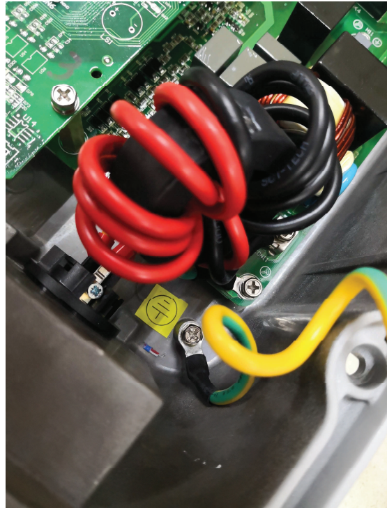
Figure 16. Earthing terminal for all modes
