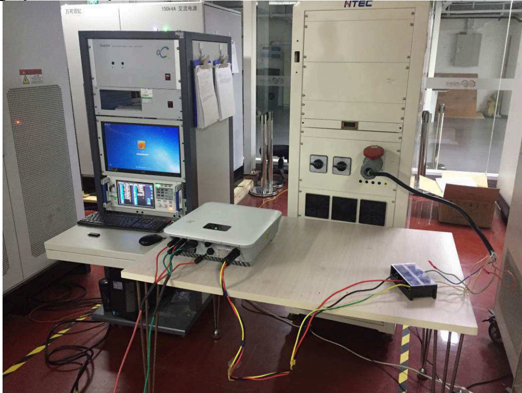
Photograph 1: Set-up for Harmonics
