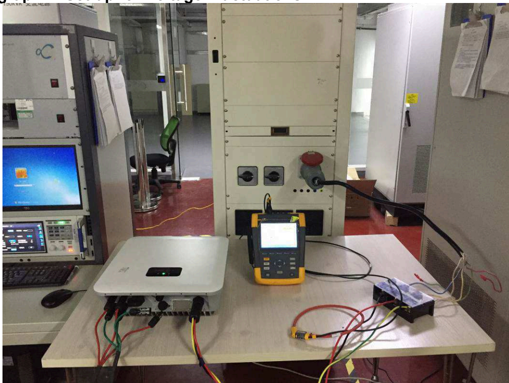
Photograph 2: Set-up for Voltage Fluctuations
