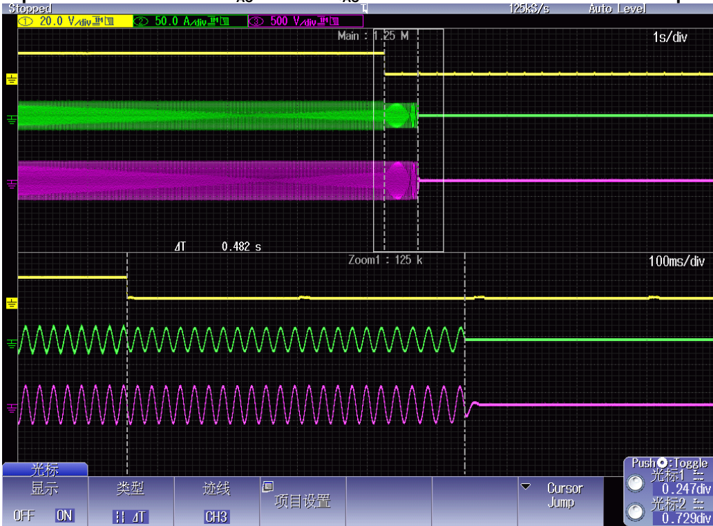
Graph of disconnection at P_{AC} 0\% and Q_{AC} -1\% reactive load and 66% nominal power
