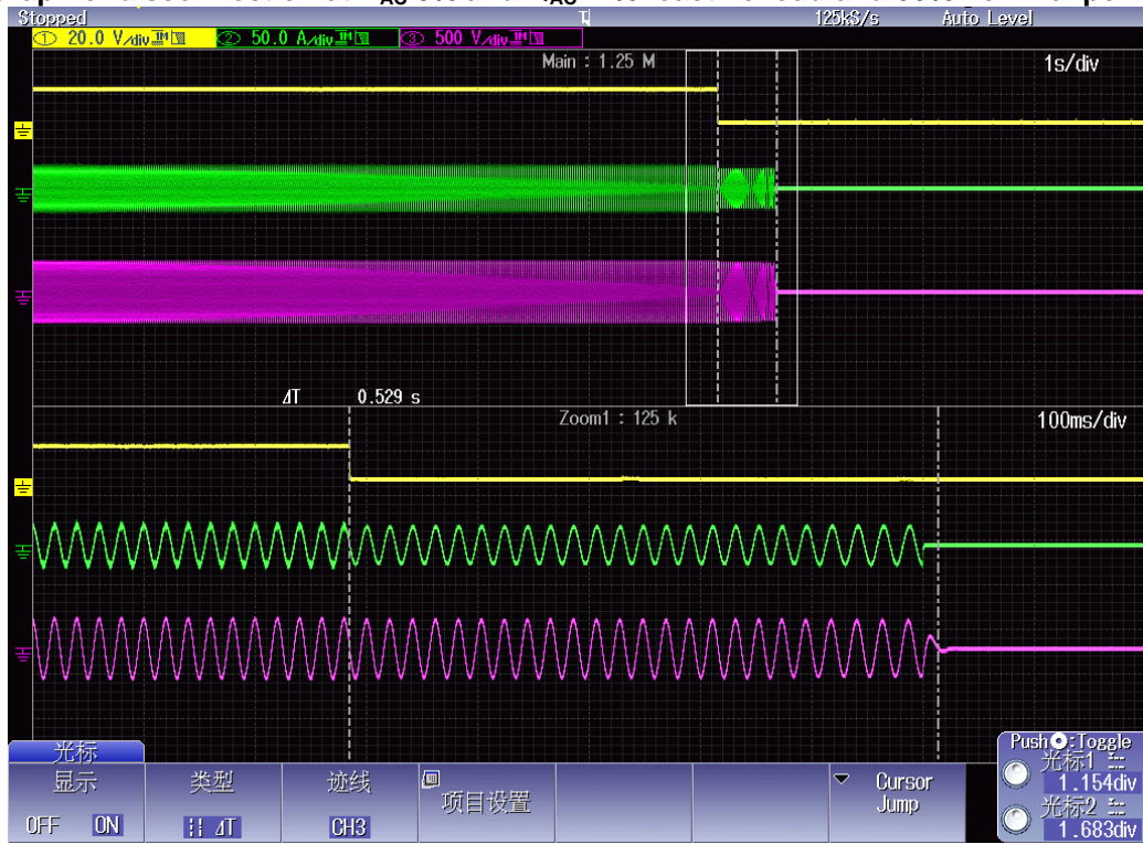
Graph of disconnection at P_{AC} 0% and Q_{AC} -2% reactive load and 66% nominal power
