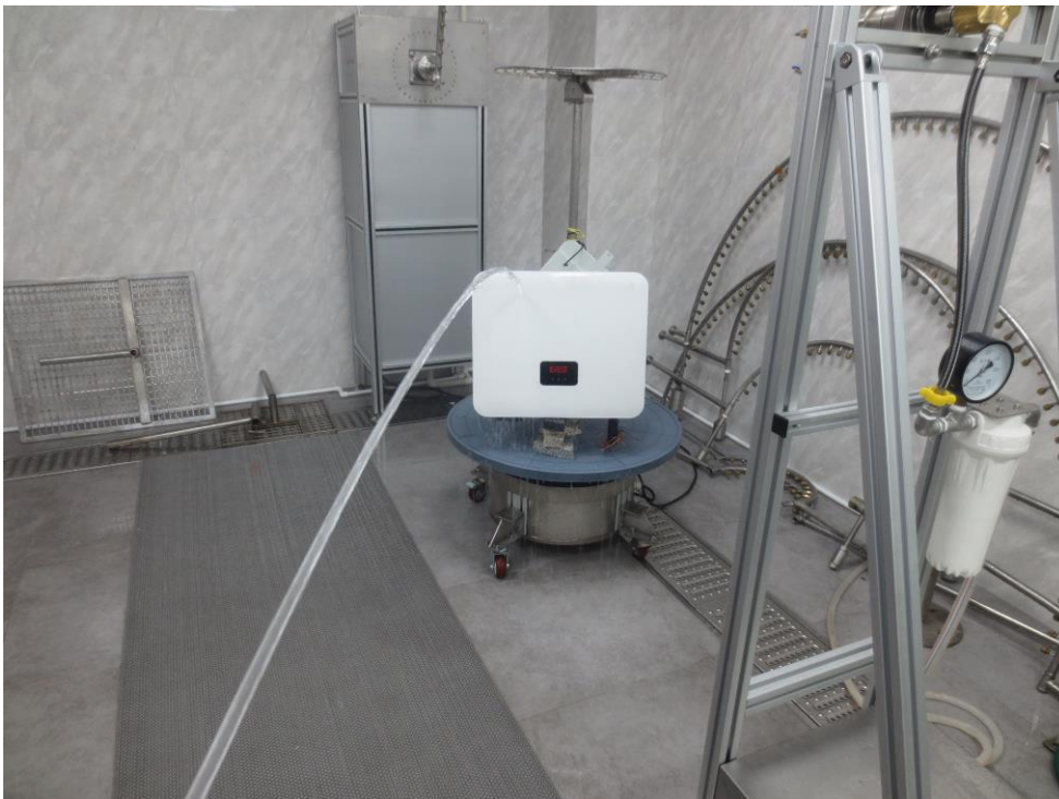
Picture during IPX5 test:
