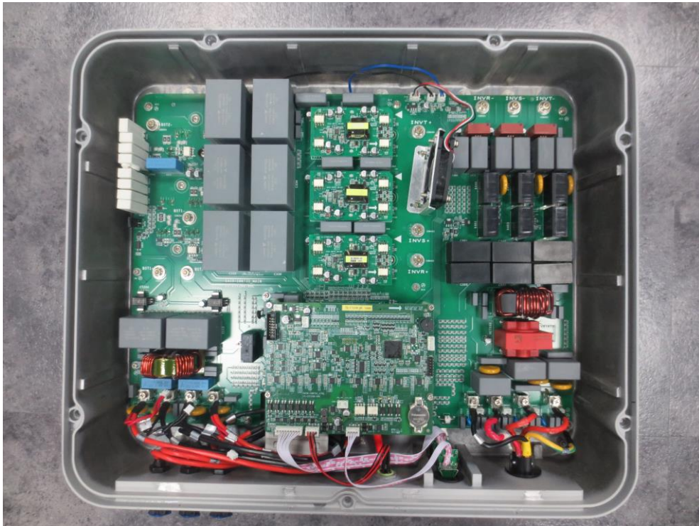
Pictures after IP65 test:
