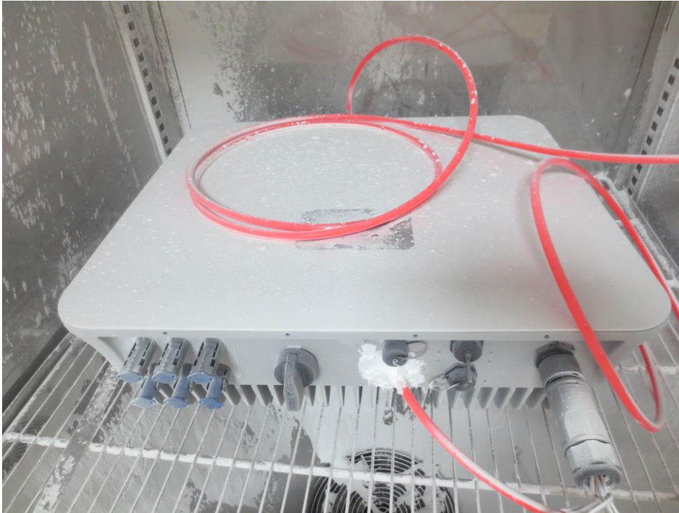
Picture during IP6X test:
