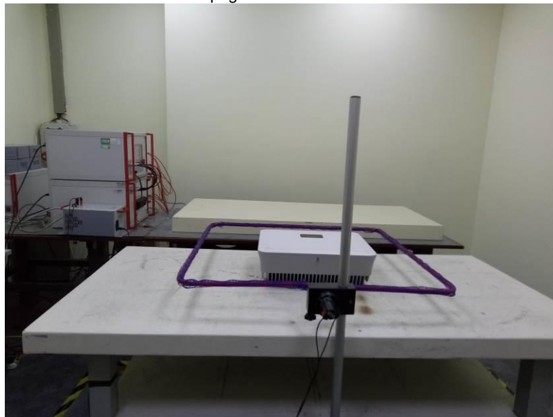
Figure 14 Power frequency magnetic field test setup
