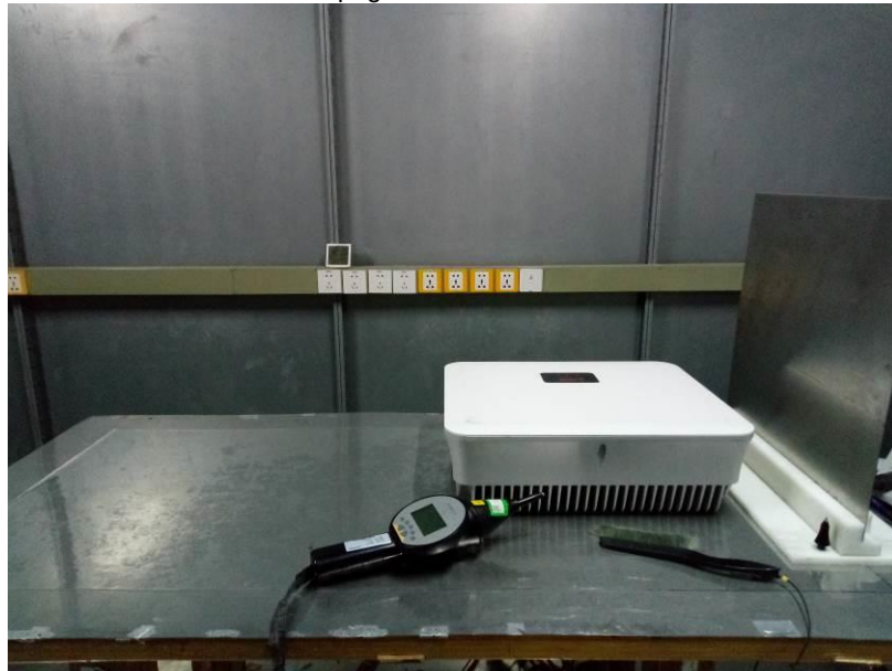
Figure 8 Electrostatic discharge test setup
