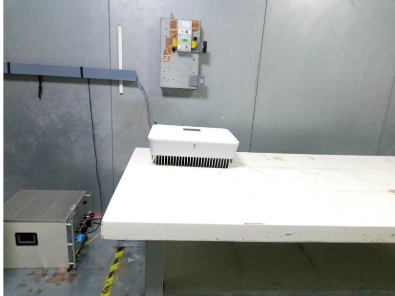
Figure 4 Conducted Emission test setup
