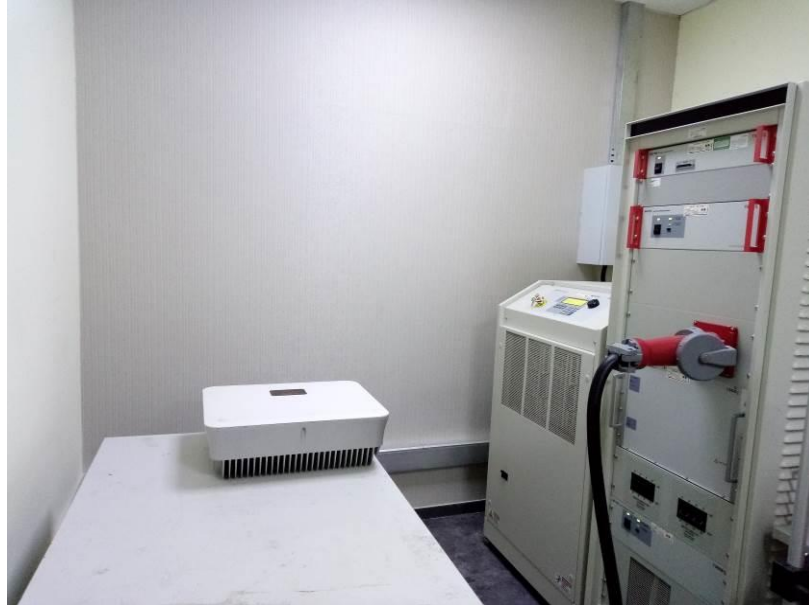
Figure 6 Harmonic current emission test setup
