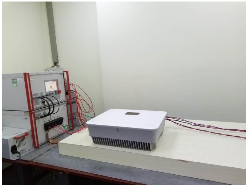
Figure 11 Electrical fast transients test setup
