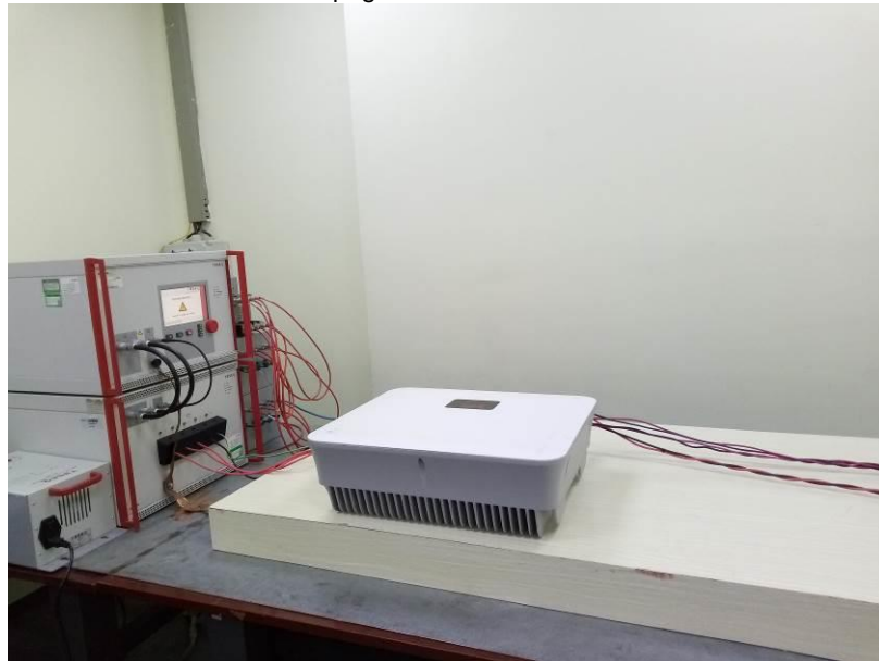
Figure 12 Surges test setup
