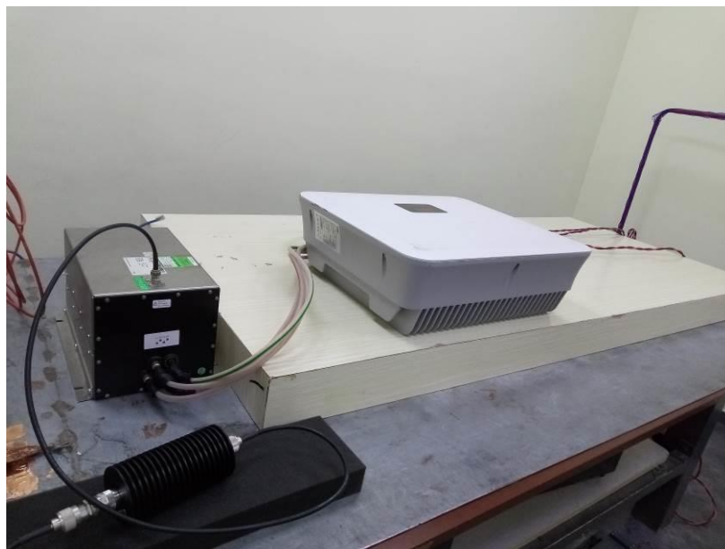
Figure 13 Radio-frequency continuous conducted test setup
