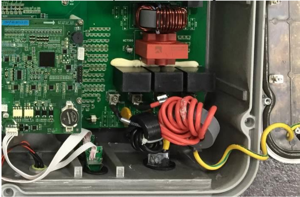
EA5KTSI / EA6KTSI / EA8KTSI / EA10KTSI / EA13KTSI / EA16KTSI AC Output and Protective Earthing
