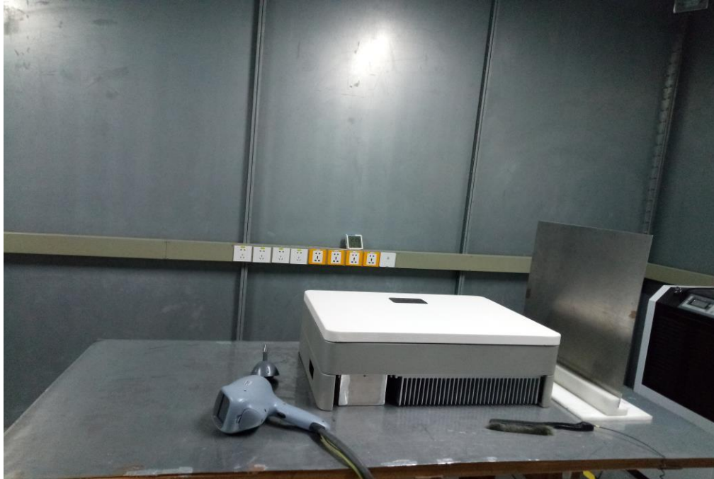
Figure 8 Electrostatic discharge test setup
