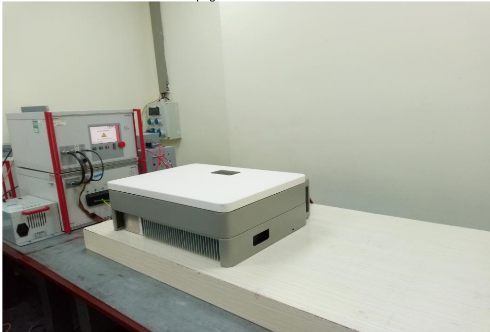
Figure 12 Surges test setup
