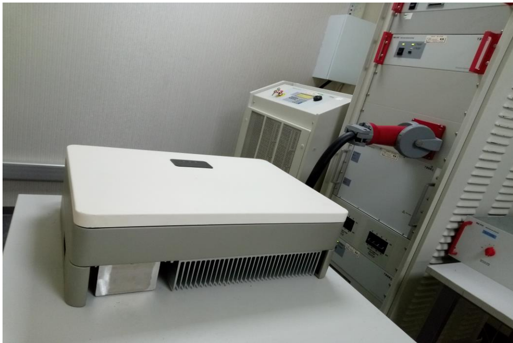
Figure 7 Voltage fluctuations and flicker test setup
