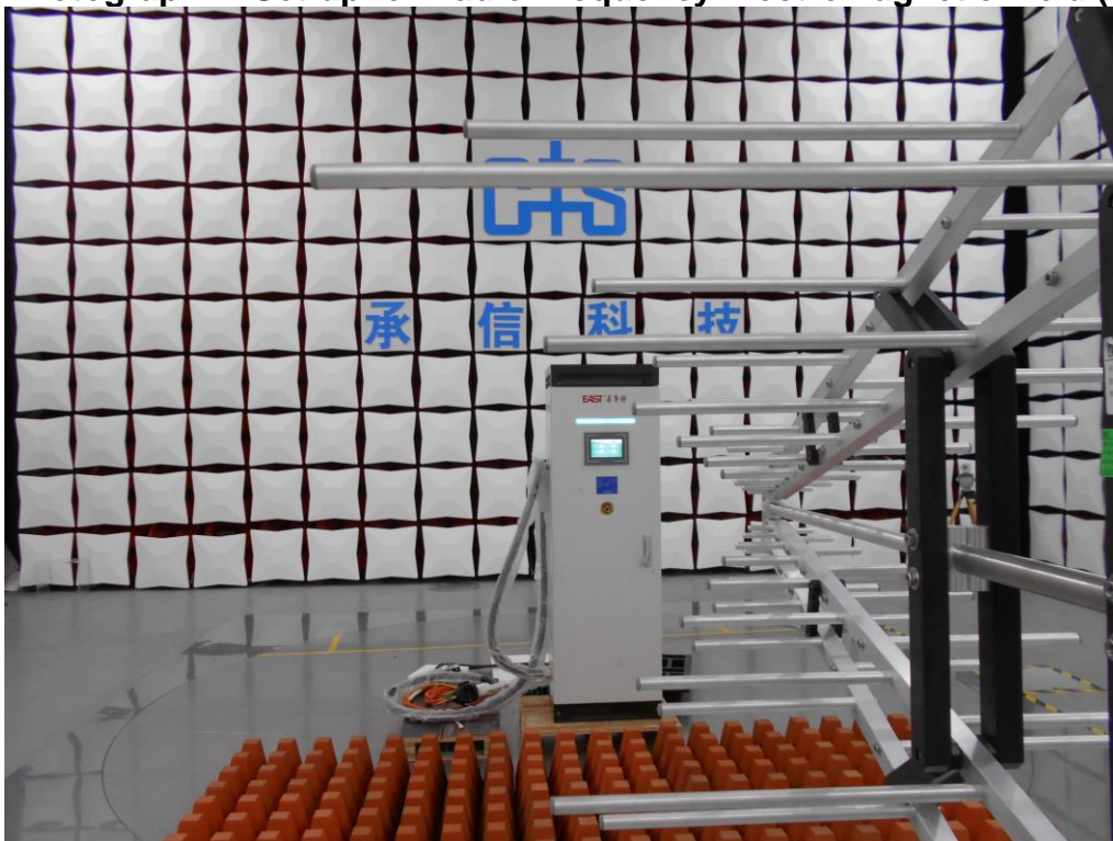
Photograph 4: Set-up for Radio Frequency Electromagnetic Field (RS)
