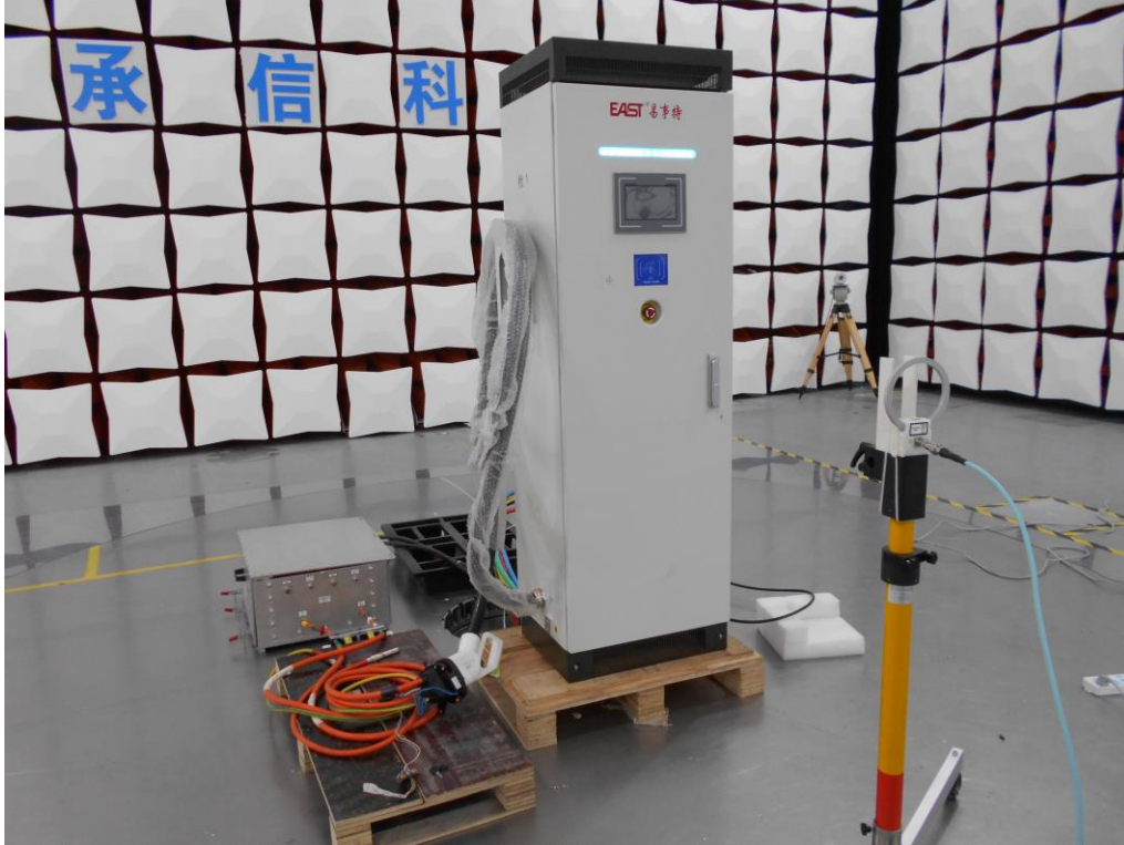
Photograph 3: Set-up for Radiated Disturbance (2KHz-185KHz)
