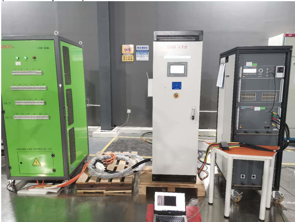
Photograph 7: Set-up for EFT (AC Power Input Port)
