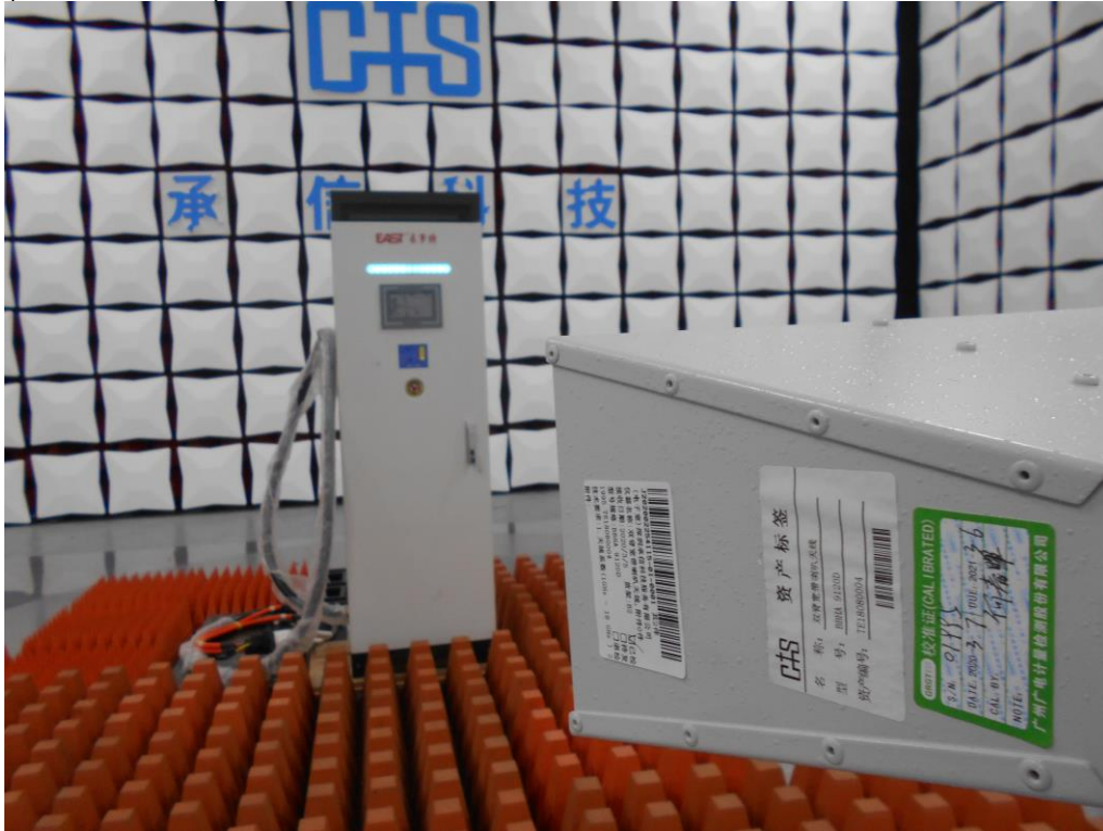
Photograph 4: Set-up for Radio Frequency Electromagnetic Field (RS)
