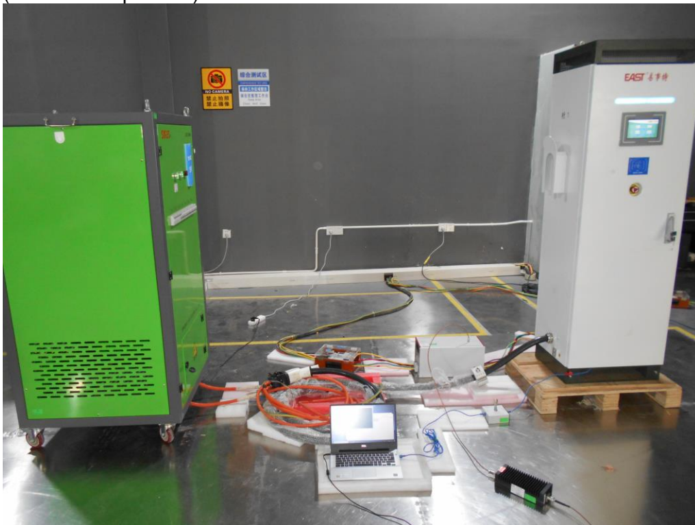
Photograph 5: Set-up for Conducted Susceptibility (CS) (AC Power Input Port)
