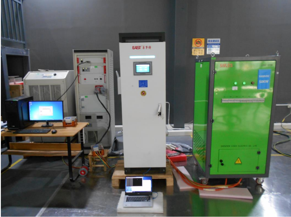
Photograph 10: Set-up for Voltage Dips and Interruptions
