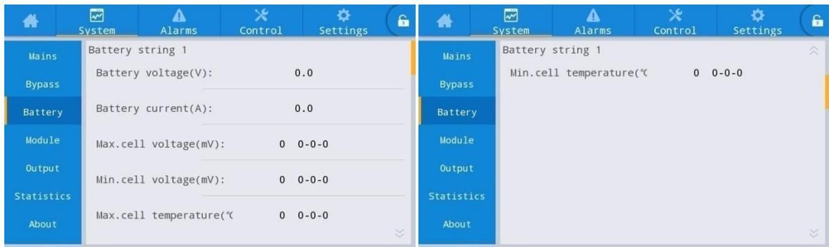
Fig. 3-9 Interface of lithium battery pack n
