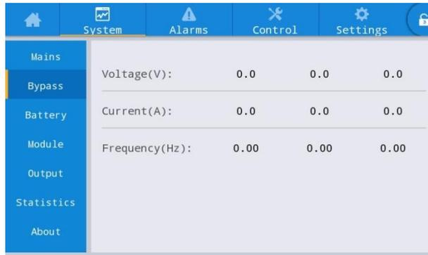
Fig. 3-6 Bypass interface
