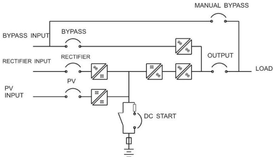
Figure 1-3 System principle
