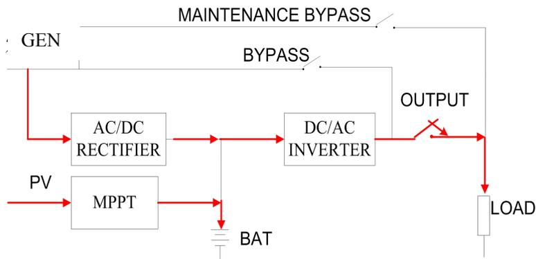
Figure 4-22 Microgrid Mode 4
