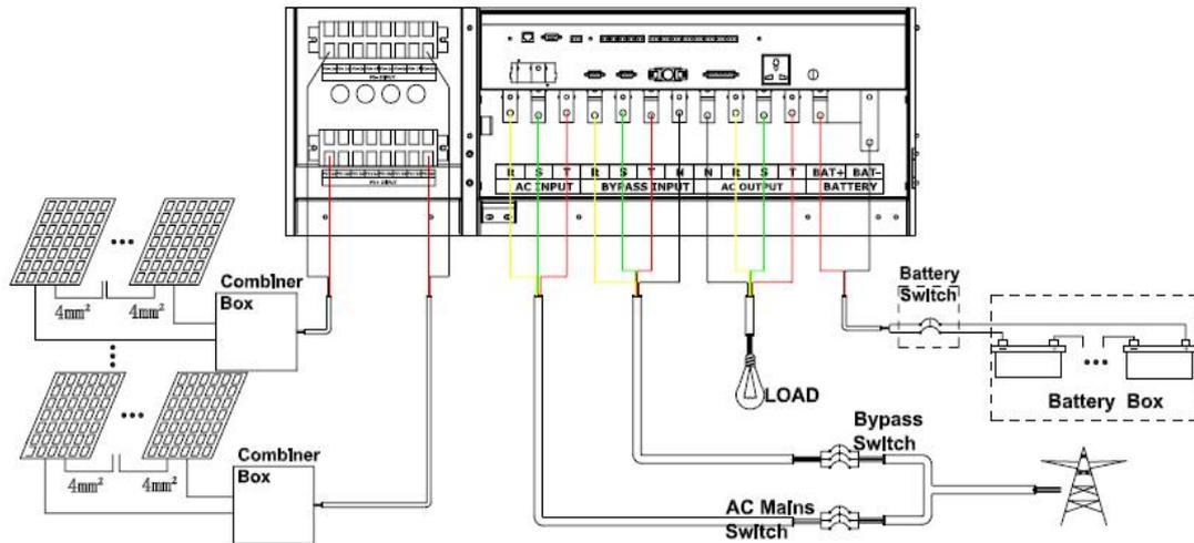
Figure 2-16 80-120 kVA Inverter Wiring in a Dual Mains System
