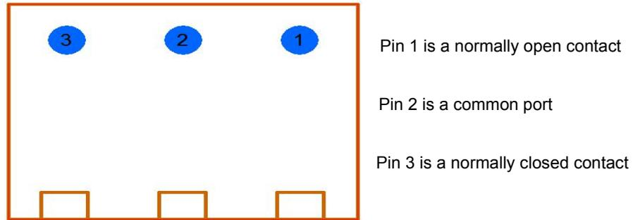
Figure 2-19 Output Dry Contact Signal Port
