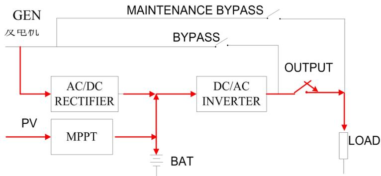
Figure 4-21 Microgrid Mode 3
