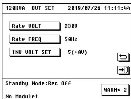
Rated voltage setting: Click “Rate VOLT” to select the appropriate rated voltage (220V/230V/240V). The rated voltage level of the inverter can be changed.
