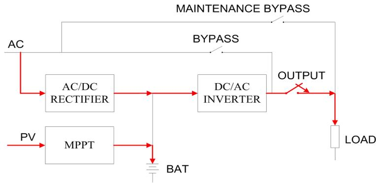
Figure 4-8 AC Charge Off Mode 2
