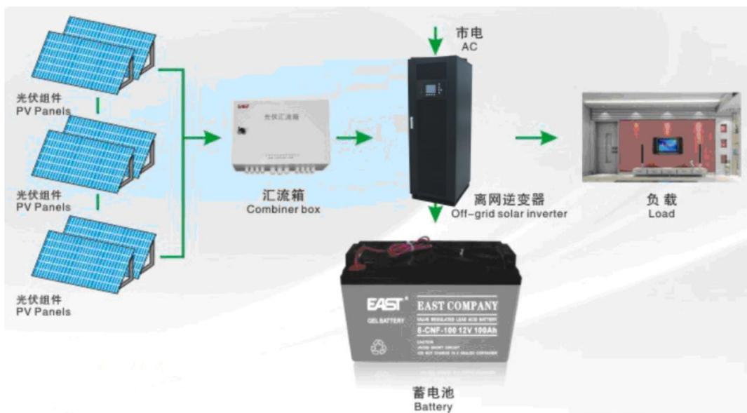
Figure 1-1 Composition of off-grid photovoltaic system
