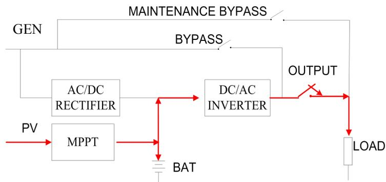
Figure 4-19 Microgrid Mode 1
