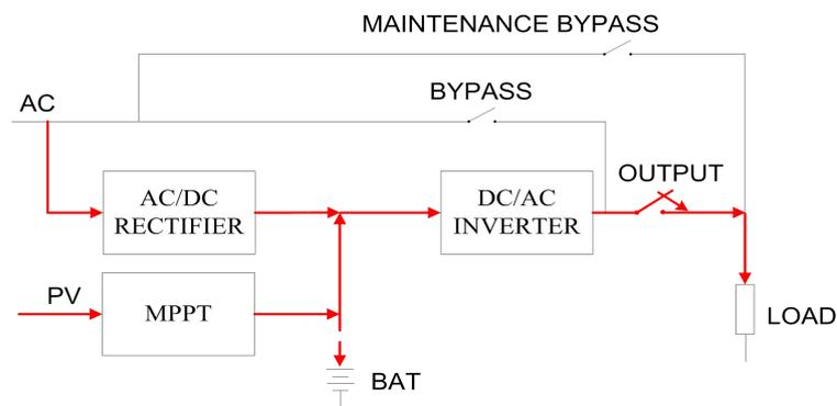
Figure 4-3 Power Supply Priority Mode 3
