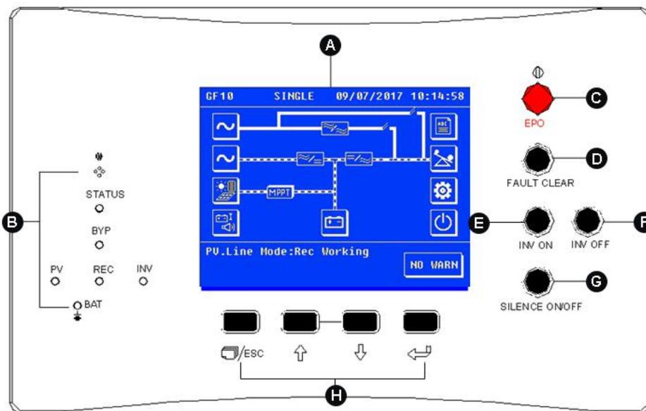
Figure 1-4 System control panel
