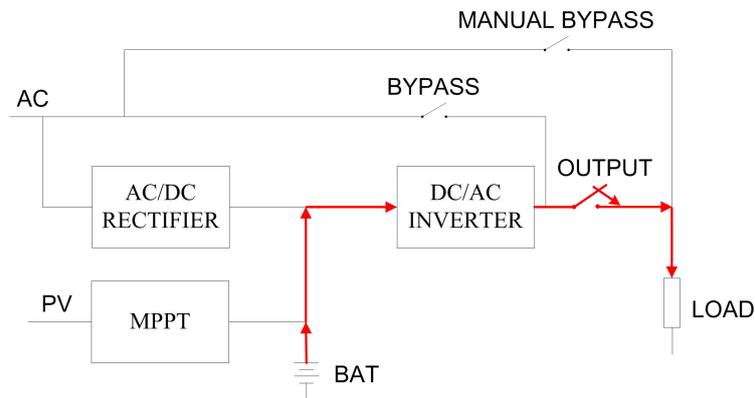
Figure 4-16 Battery Discharge Mode
