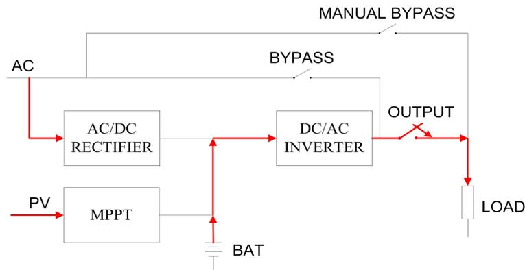
Figure 4-15 Battery Test Mode
