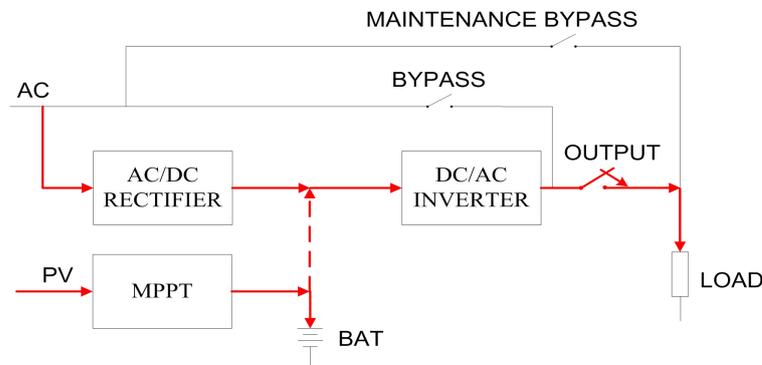
Figure 4-9 AC Charge Off Mode 3
