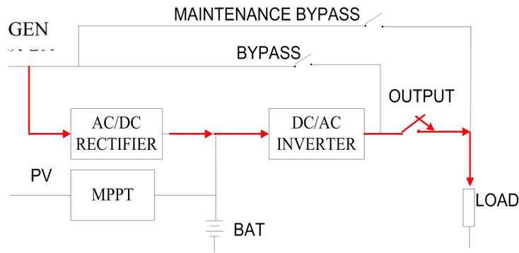
Figure 4-23 Microgrid Mode 5
