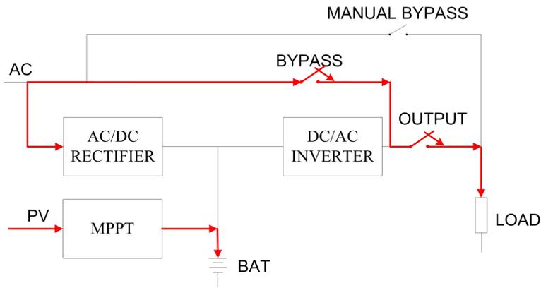
Figure 4-17 Bypass Operation Mode
