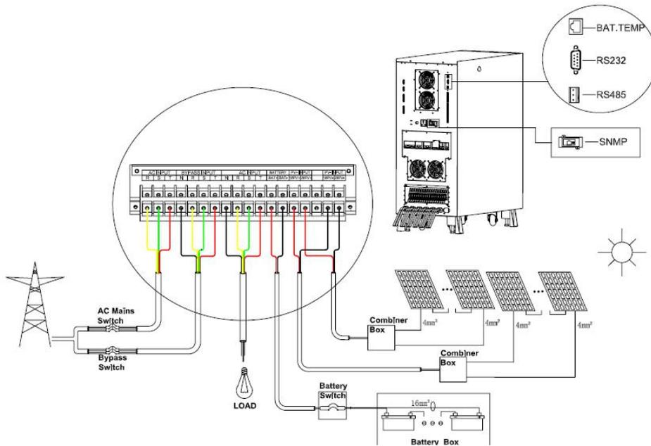
Figure 2-12 10-20 kVA inverter Wiring in a Dual Mains System
