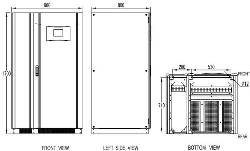
Figure 2-4 80-120 kVA Inverter Dimensions
