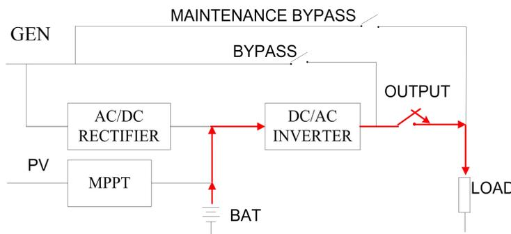
Figure 4-24 Microgrid Mode 6
