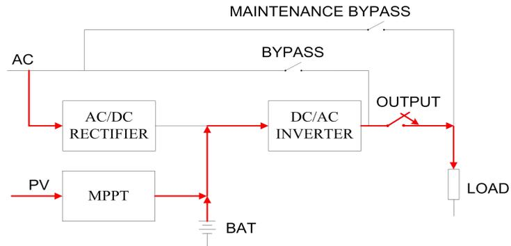
Figure 4-2 Power Supply Priority Mode 2
