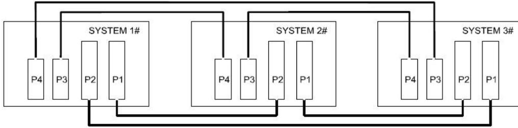
Figure 2-20 Parallel Signal Ports and Parallel System Wiring
