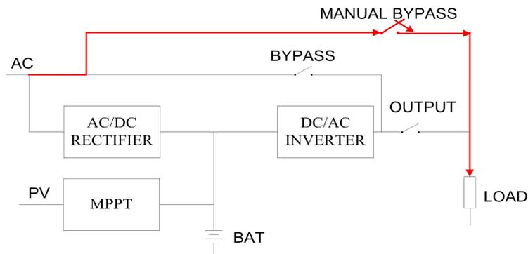
Figure 4-18 Maintenance Bypass Operation Mode
