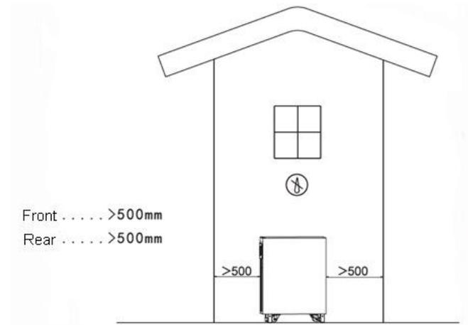
Figure 2-7 Clearance for 10-20 kVA Inverter Installation
