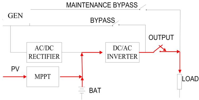
Figure 4-20 Microgrid Mode 2
