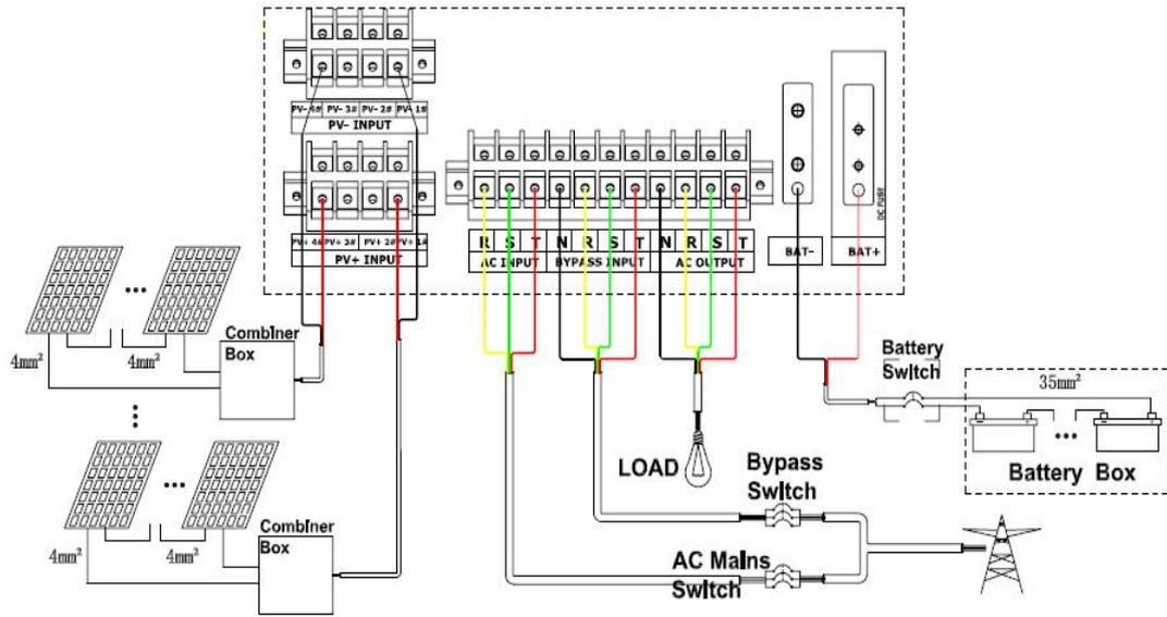
Figure 2-14 30-60 kVA Inverter Wiring in a Dual Mains System
