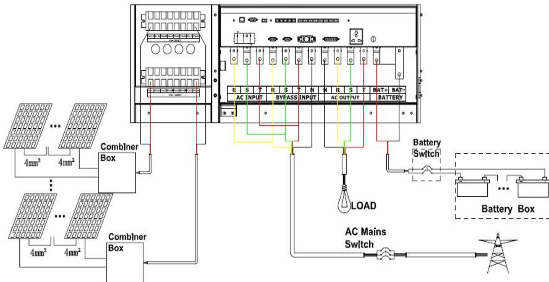
Figure 2-17 80-120 kVA Inverter Wiring in a Single Mains System
