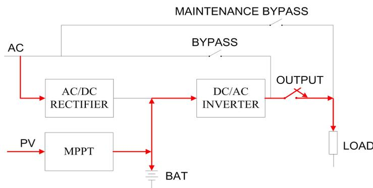
Figure 4-7 AC Charge Off Mode 1
