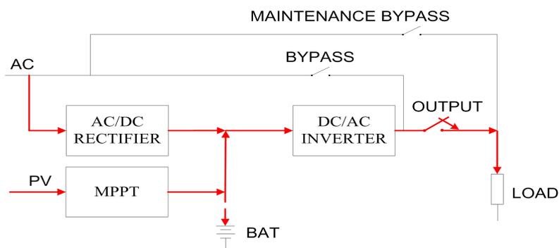
Figure 4-10 AC Charge Off Mode 4
