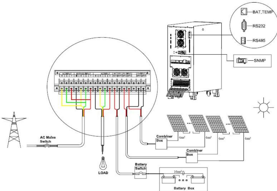
Figure 2-13 10-20 kVA Inverter Wiring In a Single Mains System
