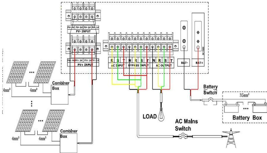
Figure 2-15 30-60 kVA Inverter Wiring in a Single Mains System
