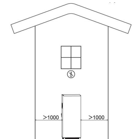
Figure 2-8 Clearance for 30-60 kVA Inverter Installation
