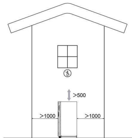
Figure 2-9 Clearance for 80-120 kVA Inverter Installation
