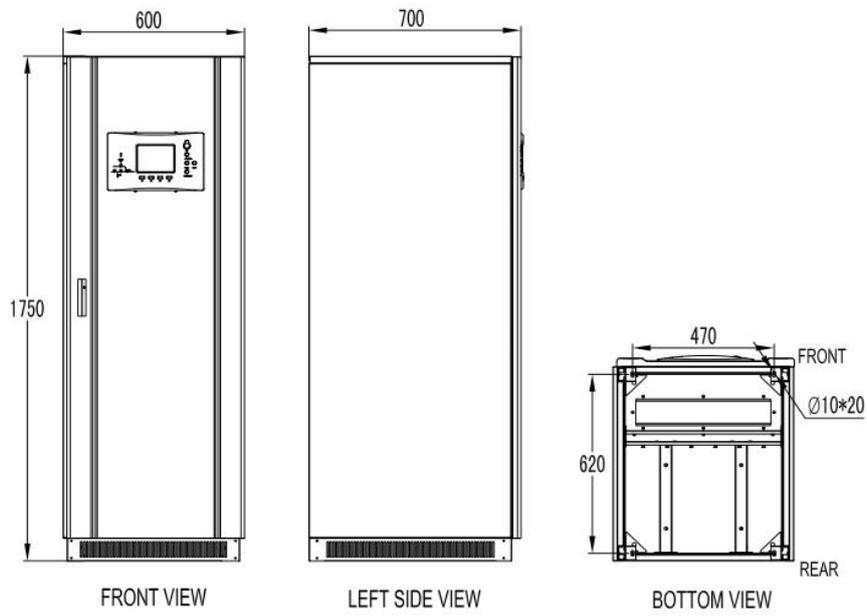
Figure 2-3 30-60 kVA Inverter Dimensions
