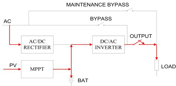
Figure 4-1 Power Supply Priority Mode 1
