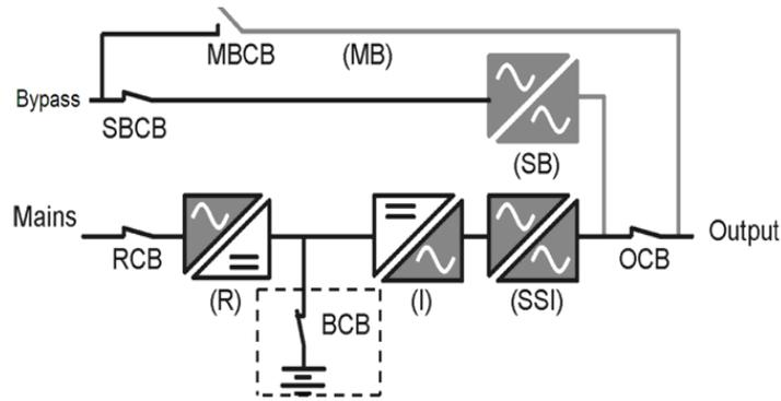
Fig. 2-2: Mains inverter power supply mode
