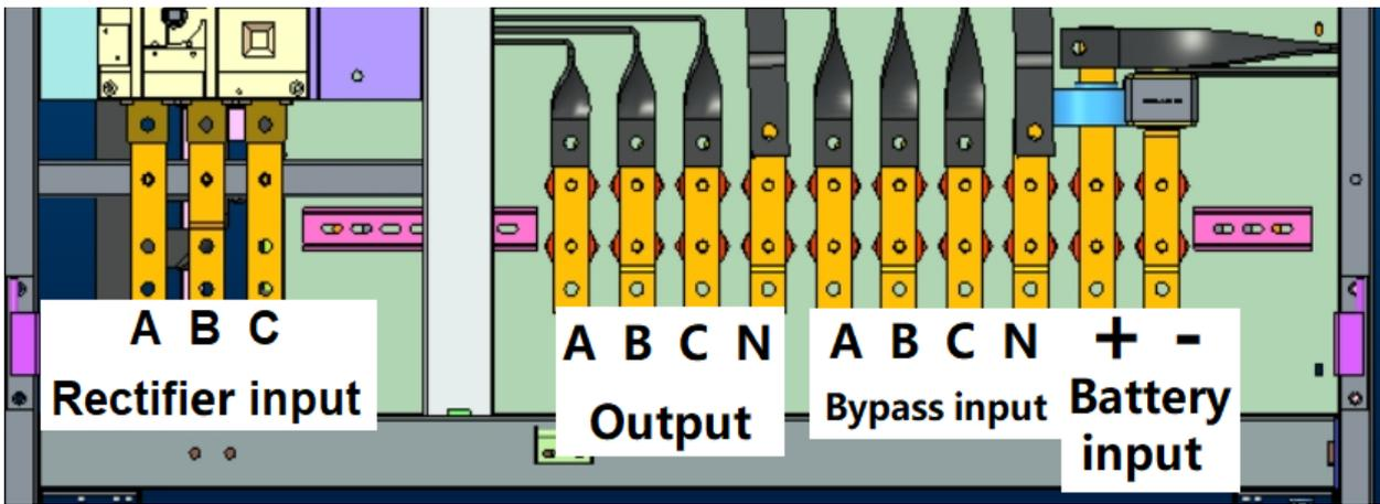
Fig. 3-36: Connection terminal of this series (200-300kVA) UPS
