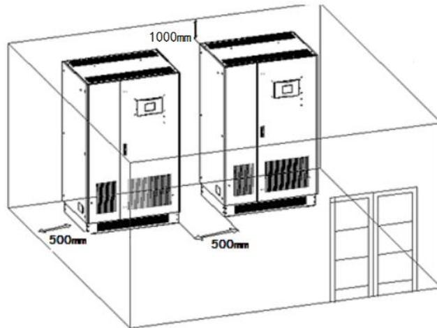
Fig. 3-11: Diagram of installation space of this series (200-300kVA) UPS (unit: mm)
