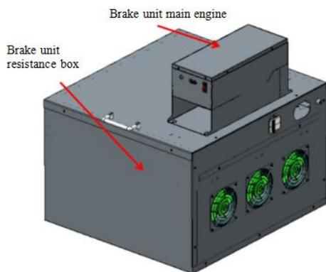
Fig. 3-26: Model of the brake unit system
