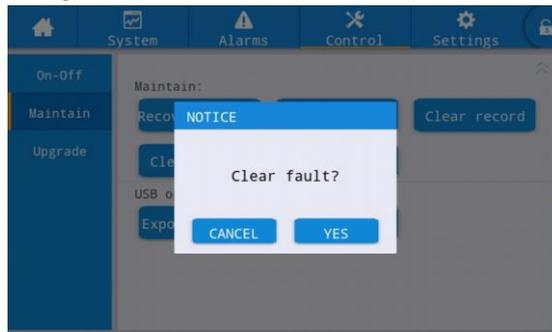
Fig. 4-11 Failure clearing confirmation interface
