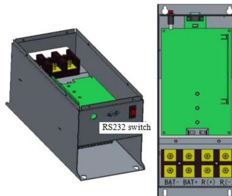
Fig. 3-27: Model of the brake unit main engine
