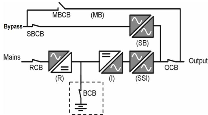
Fig. 2-1: Schematic diagram of the standard-alone system
