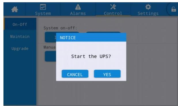
Fig. 4-3: Startup confirmation interface
