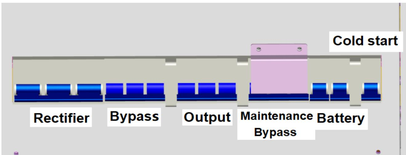
Fig. 3-31: Breaker of this series (10-40kVA) UPS
