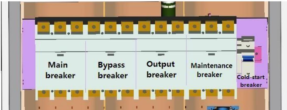
Fig. 3-33: Breaker of this series (60kVA) UPS
