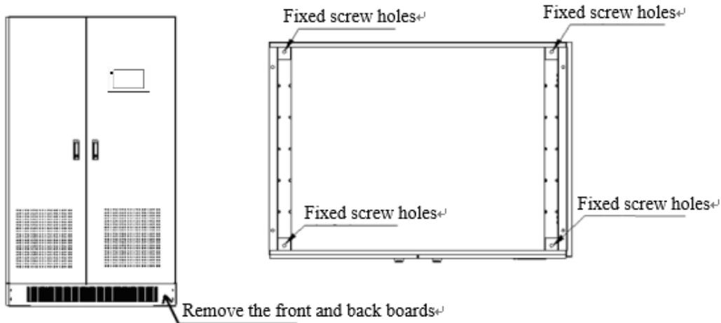
Fig. 3-6:Schematic diagram of board position Fig. 3-7:Schematic diagram of fixed screw holes on the cabinet and pallet
