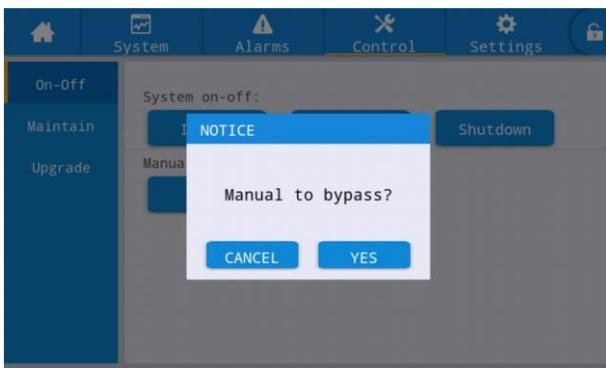
Fig. 4-9 Setting interface of manual bypass
