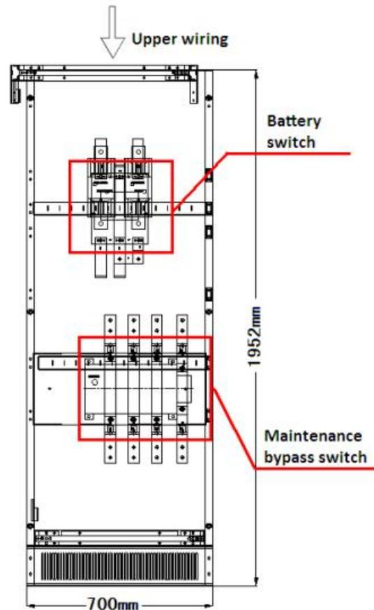
Fig. 3-24: Maintenance bypass switch integrated cabinet of this series (400-500kVA) UPS
