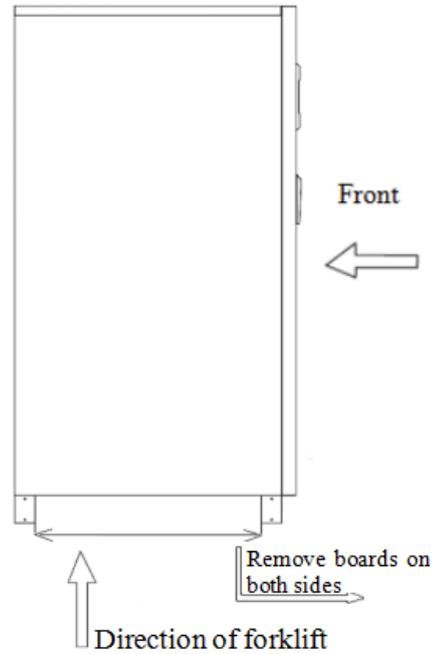
Fig. 3-14: Handling of this series (60-160kVA)
