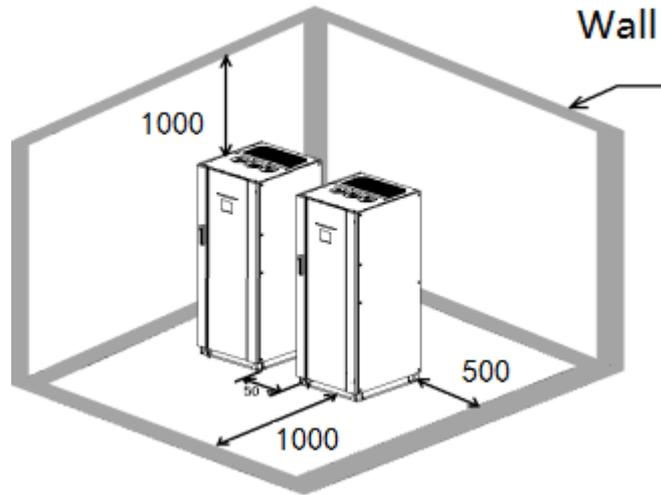
Fig. 3-10: Diagram of installation space of this series (80-160kVA) UPS (unit: mm)
