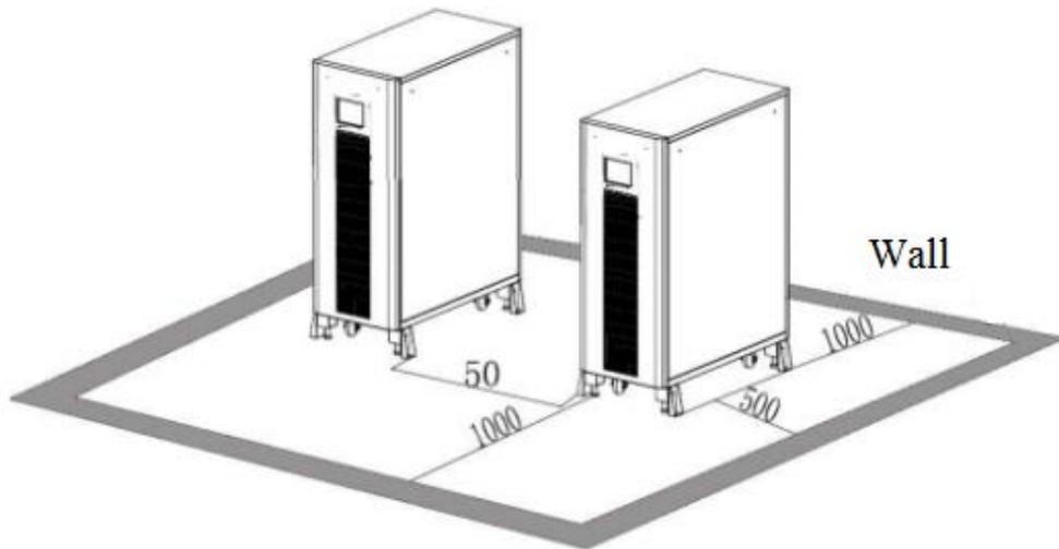
Fig. 3-8: Diagram of installation space of this series (10-40kVA) UPS (unit: mm)
