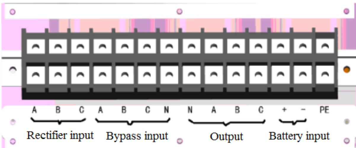
Fig. 3-30: Connection terminal of this series (10-40kVA) UPS
