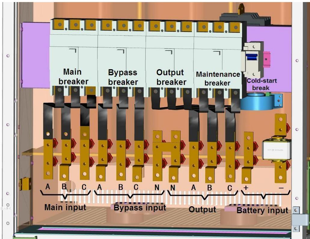
Fig. 3-34: Breaker of Connection terminal and this series (80-120kVA) UPS
