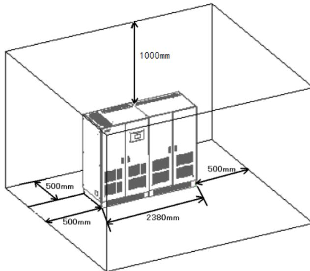
Fig. 3-12: Diagram of installation space of This series (400-500kVA) UPS (unit: mm)
