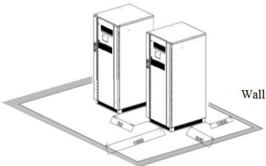
Fig. 3-9: Diagram of installation space of this series (60kVA) UPS (unit: mm)
