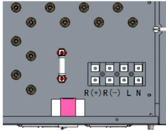
Fig. 3-28: Connection terminal of the brake unit main engine      Fig. 3-29: Connection terminal of the brake unit resistance box
