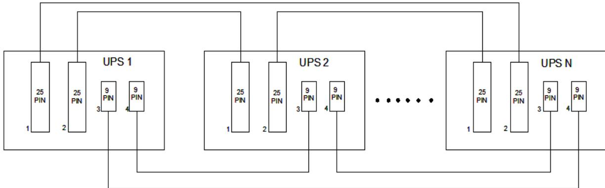
Fig. 3-42: Schematic diagram of parallel signal line connection
