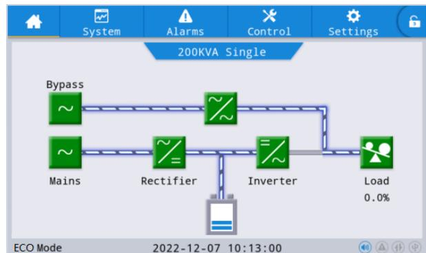
Fig. 4-10 Effective energy flow chart of manual bypass
