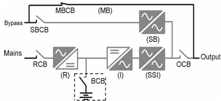
Fig. 2-5 Maintenance bypass mode
