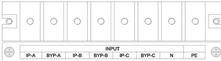
Fig.3-5 connections terminals for 40-60kVA model
