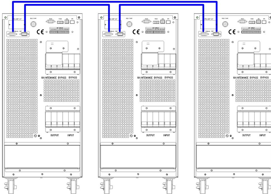
Fig.5-6 Parallel connection
