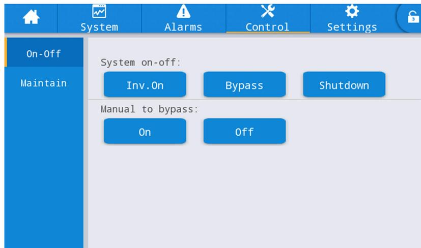
Fig. 5.2 Operation for switching the UPS into bypass mode
