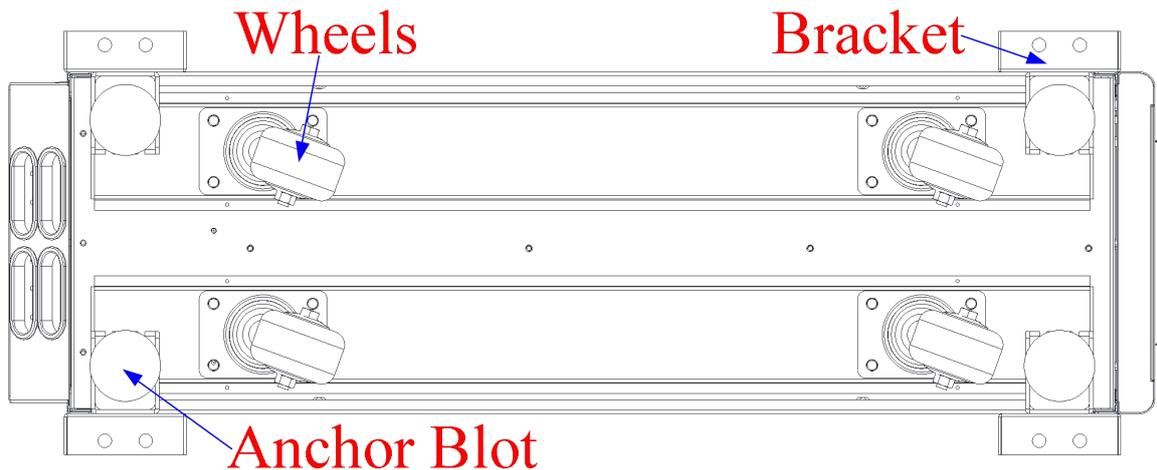
Fig.3-1 Supporting structure (Bottom view)
