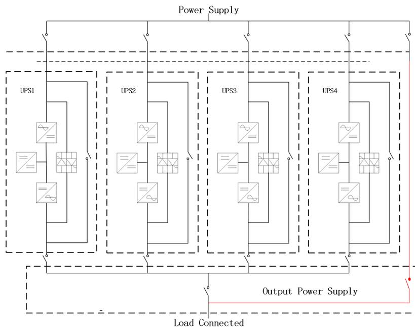
Fig. 5-5 Parallel diagram
