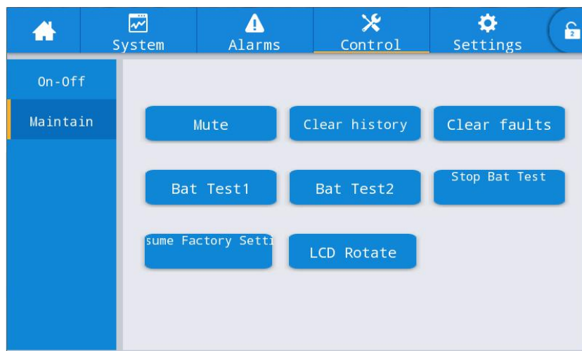
Fig. 5-4 Battery maintenance page
