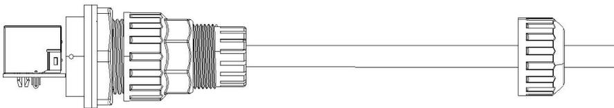
Twist the connection nut clockwise to the RJ45 connector with a recommended torque of 2N·m.
