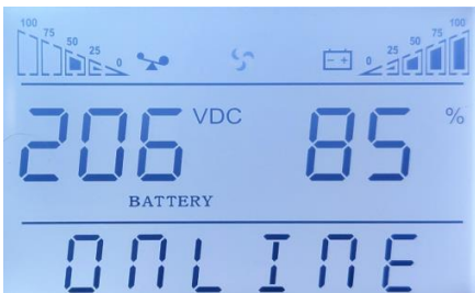
Page 6: Display UPS battery voltage, battery capacity percentage
