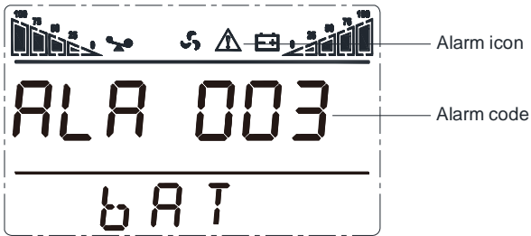
Tower UPS LCD display in alarm mode
