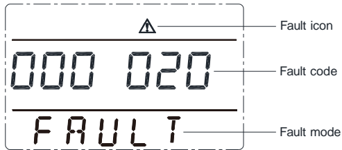
Tower UPS LCD display in fault mode
