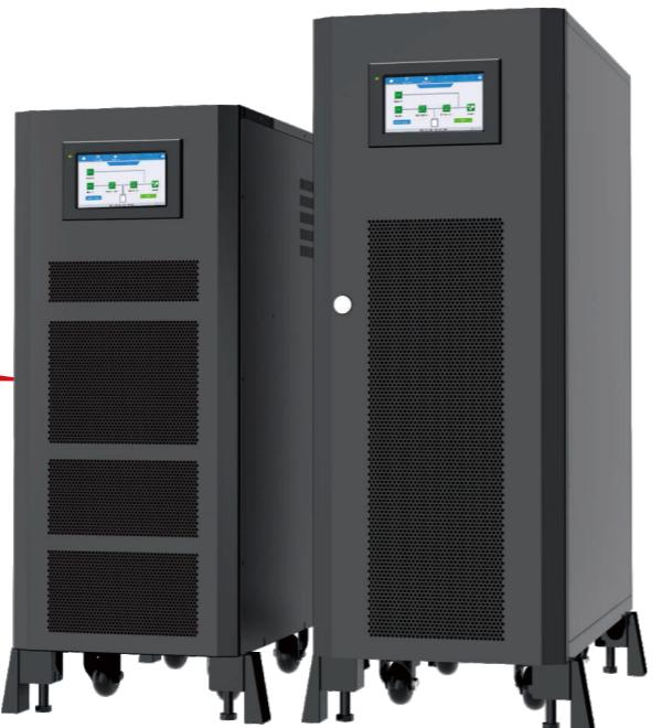
This series is an online dual-conversion UPS, a 2-level topology design with bidirectional rectifier and inverter, which supports regenerative load, with no need for an extra Dynamic Braking Resistor (DBR), especially for industrial loads like motors, lifts, and laser cutting machines.
