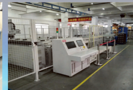
Online lithium cell multi-grade sorting test system
