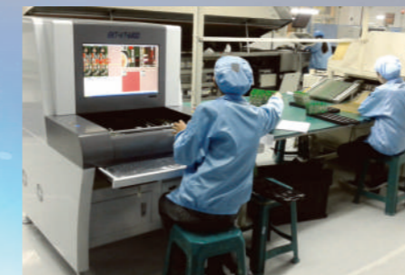
Multi-temperature zone hot reflow soldering and AOI automated optical inspection system
